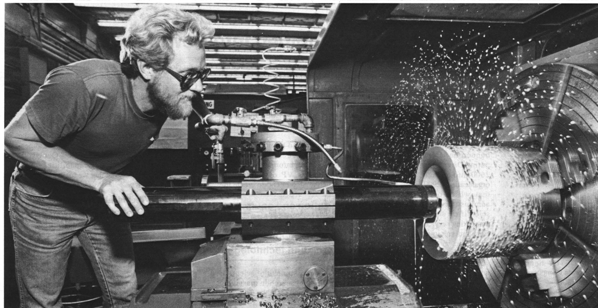
SPLASHING WATER-BASED coolant assists the process as Tim Mitchell (7482) turns a part in the 32-inch lathe.
